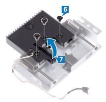
**8** Pull the clip on the retractable-camera assembly, and rotate the camera and camera bracket along with the camera cable, off the retractable-camera assembly.
