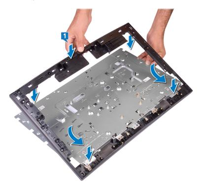
2 Replace the 13 screws (M3x5 black) that secure the middle frame to the display-assembly base.
