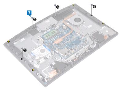
8 Remove the four jig screws from the display panel.
