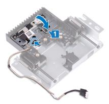
2 Align the screw holes on the camera-assembly cover with the screw holes on the retractable-camera assembly.
