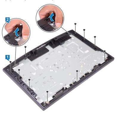
Lift and slide the display-assembly base off the middle frame.
