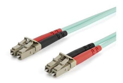
This OM3 LC to LC Multimode Duplex Fiber Optic Patch cable features 50/125 micron fiber and supports high-bandwidth data transmission over a 10 Gigabit Ethernet connection.
