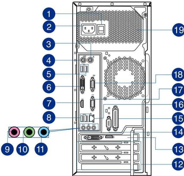
**1 Voltage selector.** Use this switch to select the appropriate system input voltage according to the voltage supply in your area. If the voltage supply in your area is 100-127V~, set the switch to 115V~. If the voltage supply in your area is 200-240V~, set the switch to 230V~.
