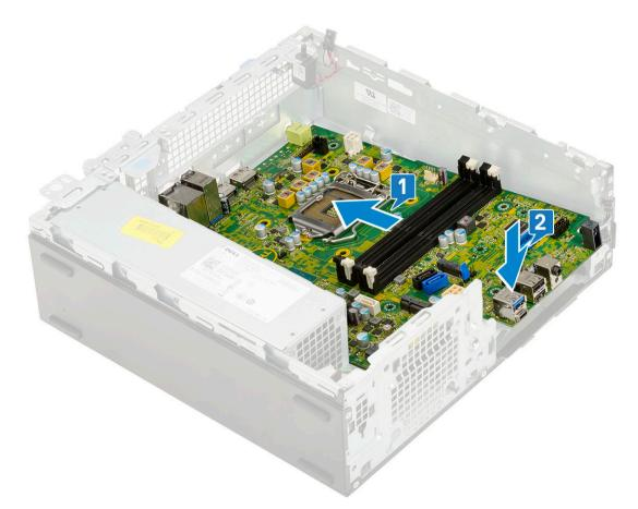
3 Replace the standoff single (#6-32) screw, the single screw used as a mounting point for M.2 SSD drive and the 5 screws that secure the system board to the system [1, 2, 3][1,2].
