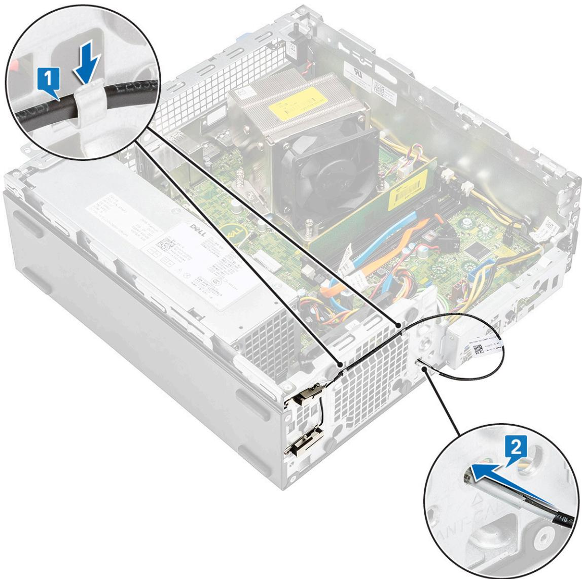
g Remove the plastic tube from internal antenna cable.
