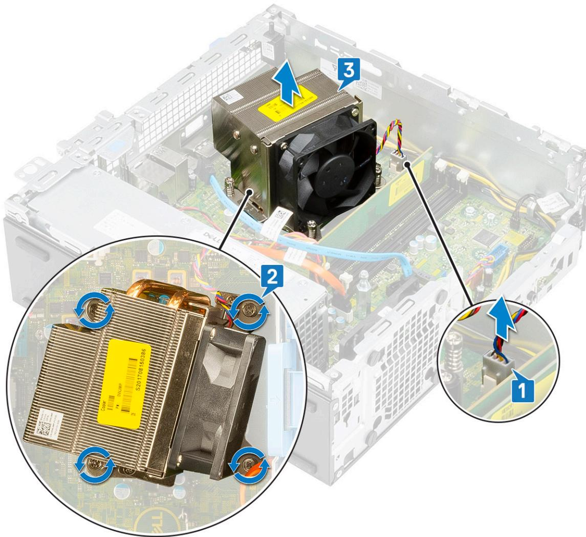
4 To remove the heat sink fan:
