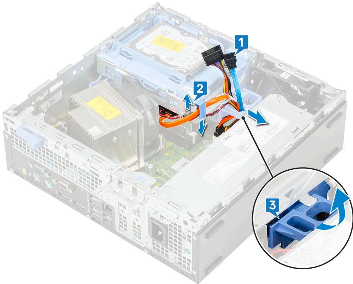
5 Remove the hard drive and optical drive module:
