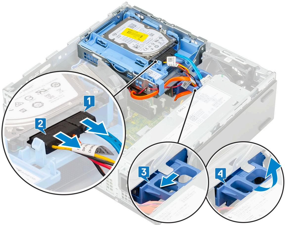
d Disconnect the optical drive data cable and optical drive power cable from the connectors on the optical drive [1, 2] and lower the hard drive and optical module until it is seated [3].
