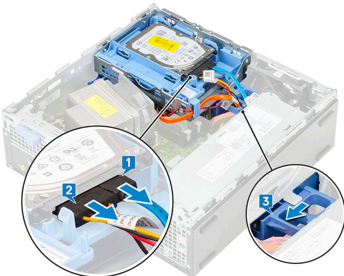
c Unroute the hard drive cables [1] and optical drive cables [2] through the retention clip and HDD-ODD release tab respectively.
