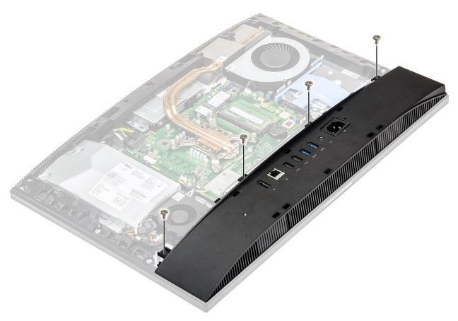
4 Pry and lift the base cover off the middle frame.
