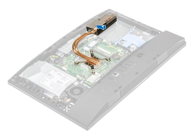
2 Tighten the five captive screws in a sequential order [1,2,3,4,5] to secure the heat sink to the system board and display assembly base..
