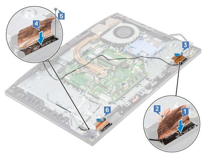
d Route the antenna cables through the routing guides on the display assembly base [1,2].
