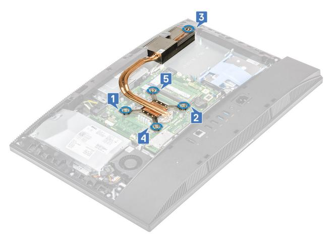
4 Lift the heat sink off the system board and display assembly base .
