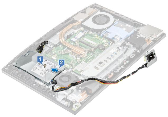
b Slide the PSU, and lift it away from the chassis .
