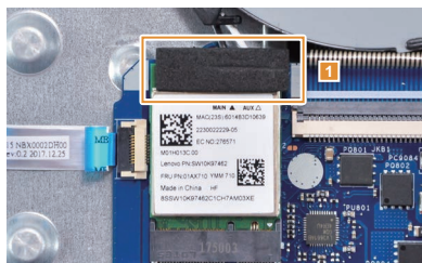
Figure 6. Removal steps of PCI Express Mini Card for wireless LAN
