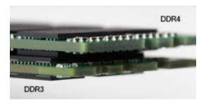
Figure 2. Thickness difference
