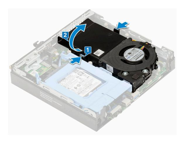
4 Disconnect the speaker cable and heat sink blower cable from the connectors on the system board.
