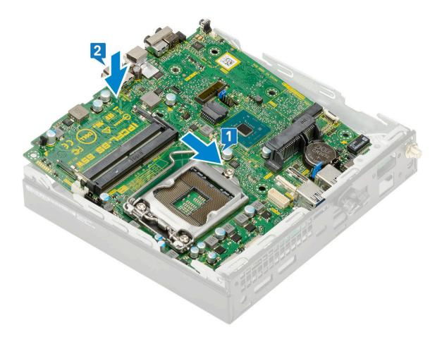
c Replace the two (M3x4) screws [1] and three (6-32x5.4) screws [2] to secure the system board to the system.
