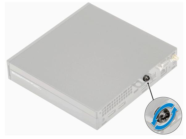
b Slide the side cover towards the front of the system and lift the cover to remove from the system.
