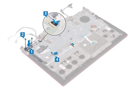
5 Adhere the tape that secures the fingerprint-reader board and the power-button board to the palm-rest assembly.
