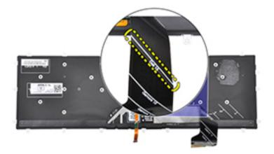
2 Gently fold the keyboard cable with the end aligned at the fold line as shown in the image. Once folded correctly, the right edge of the keyboard cable should be lined up next to the line indicated on the palm-rest assembly.
