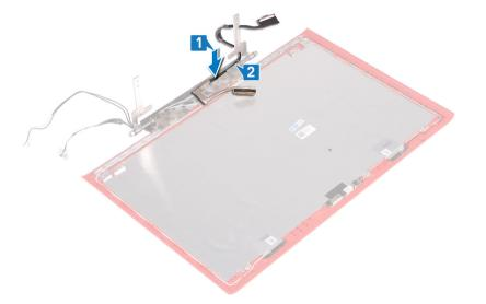
3 Adhere the tape that secures the display cable to the display back-cover and antenna assembly.
