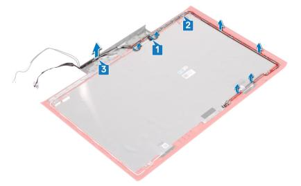
3 After performing the above steps, we are left with the display back-cover and antenna assembly.
