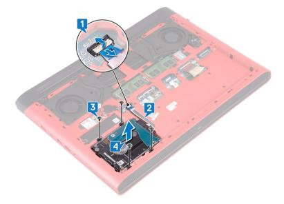
5 Disconnect the interposer from the hard-drive assembly.
