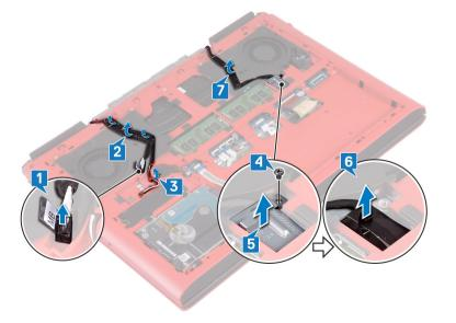
8 Open the latch and disconnect the power-button board cable from the system board.
