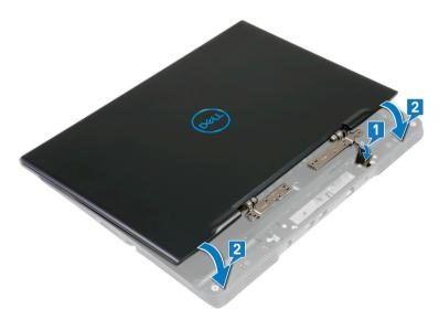
3 Replace the eight screws (M2x4) that secure the left and right hinges to the palm-rest assembly.
