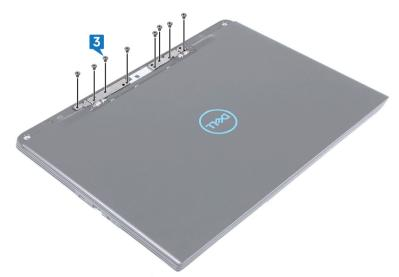
4 Align the hinge cover with the slots on the palm-rest assembly and press to secure the hinge cover.
