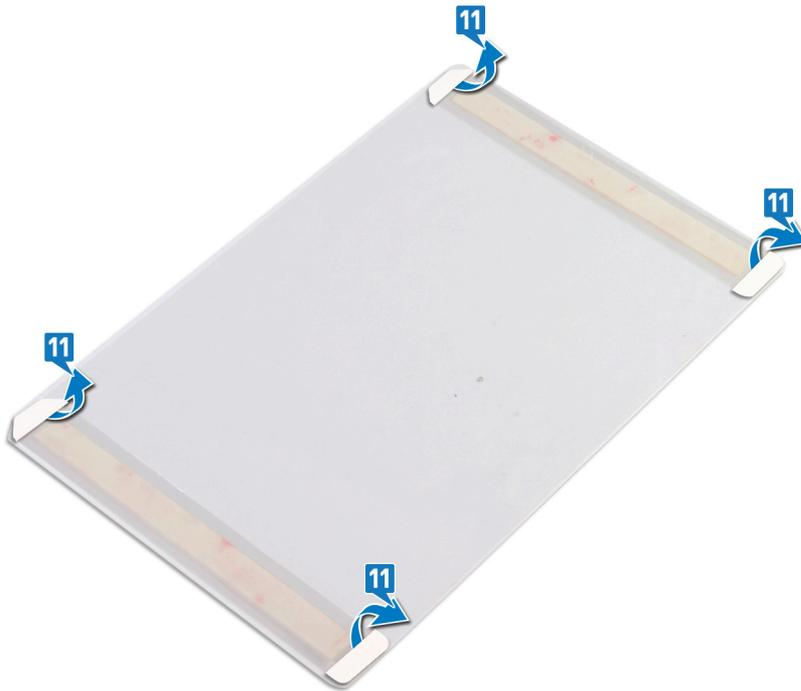
12 Adhere the pressure film on the display panel.
