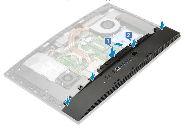
3 Replace the four screws (M3x5) that secure the base cover to the display assembly base.
