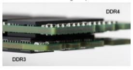
Figure 2. Thickness difference
