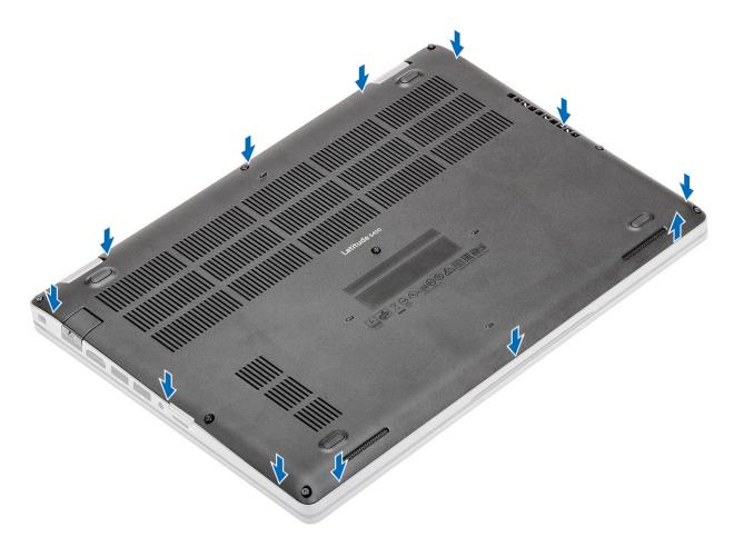
3 Tighten the eight captive screws to secure the base cover to the computer.
