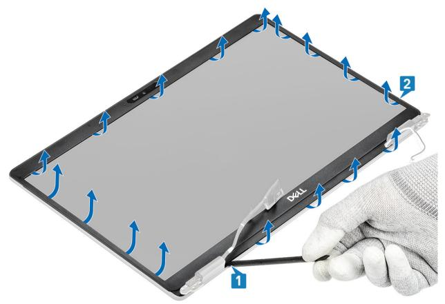
3 Lift the display bezel from the display assembly.
