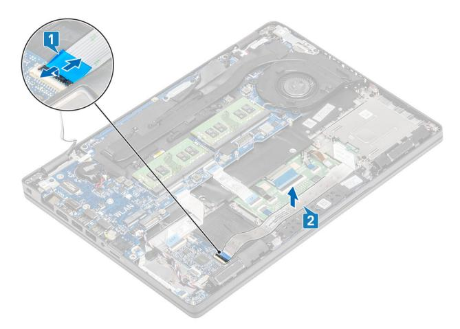
3 Open the latch and disconnect the touchpad button board cable from the connector on the touchpad board [1, 2].
