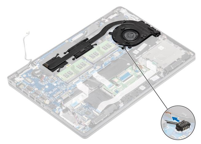
2 Remove the six (M2x3) screws that secure the heatsink assembly to the system board [1].
