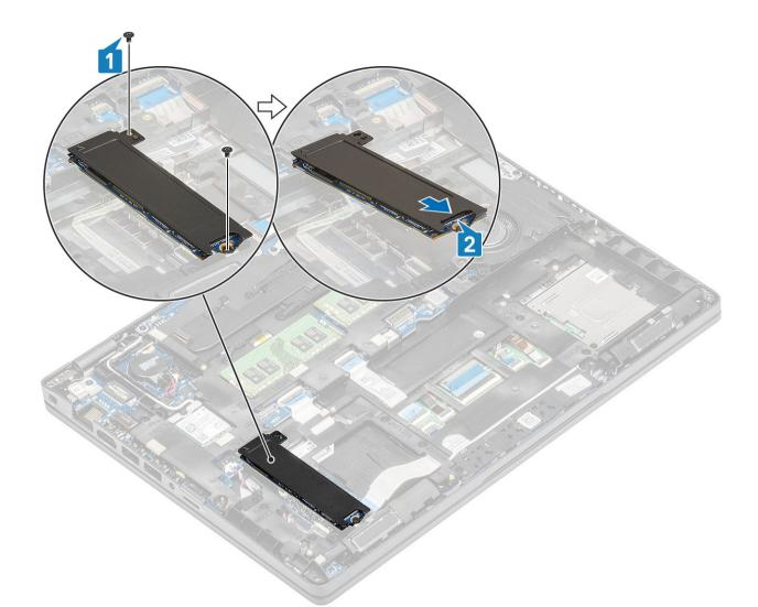
3 Remove the SSD of the SSD thermal plate.
