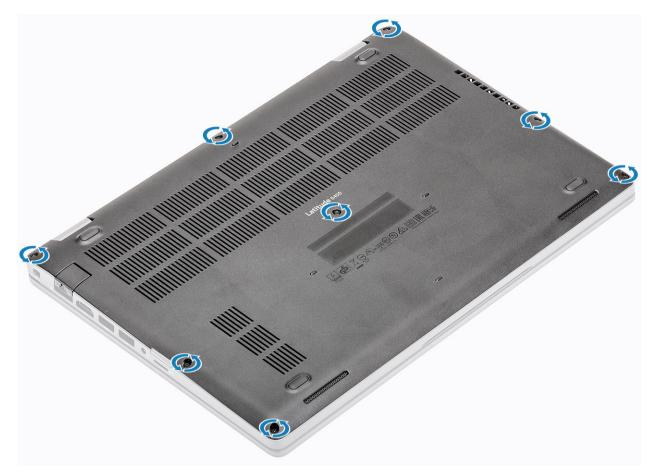
2 Using a plastic scribe [1], pry the base cover from the top-left corner and continue to work on the sides to open the base cover [2].
