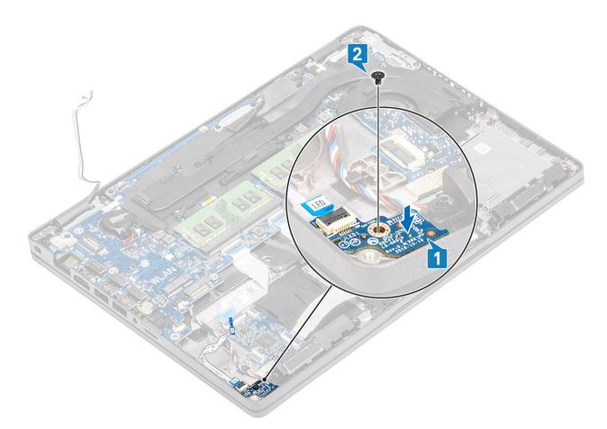
3 Connect the LED board cable to the connector on the system board and route the LED board cable [1, 2].
