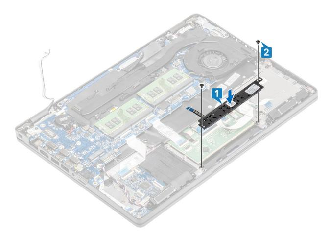
3 Connect the touchpad button board cable to the connector on the touchpad board [1, 2].
