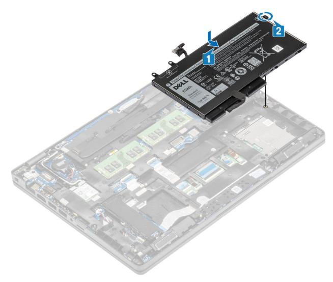
3 Connect the battery cable to the connector on the system board.
