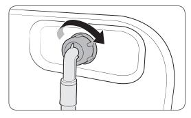
Connect the water hose to the water tap, and then turn the connector clockwise as shown.
