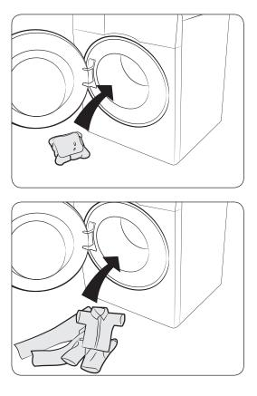
**1.** Put the capsule in the bottom of the empty drum towards the rear.
