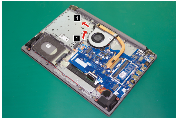
Figure 15. Release the antenna cables
