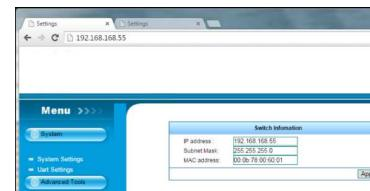
**Step 3:** Use a web browser to access the unit (TX:192.168.168.55, RX:192.168.168.56). Click the **System** menu and setup the required IP address, subnet mask, and MAC address as mentioned above. **It is highly recommended to label the units with this setting. If you ever forget this setting you may have to reset the units to factory default values!**
