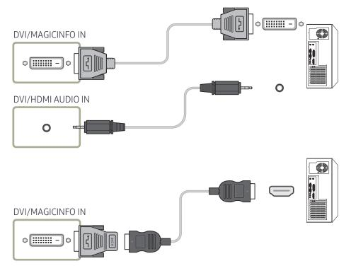
You can use the DVI port on the product as an HDMI port by using a DVI-HDMI adapter. Audio is not available if the DVI port on the product is connected to the HDMI port on the PC using a DVI-HDMI adapter.
