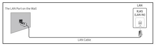
If you have a Dynamic Network, you should use an ADSL modem or router that supports the Dynamic Host Configuration Protocol (DHCP). Modems and routers that support DHCP automatically provide the IP address, subnet mask, gateway, and DNS values your product needs to access the Internet so you do not have to enter them manually. Most home networks are Dynamic Networks.
