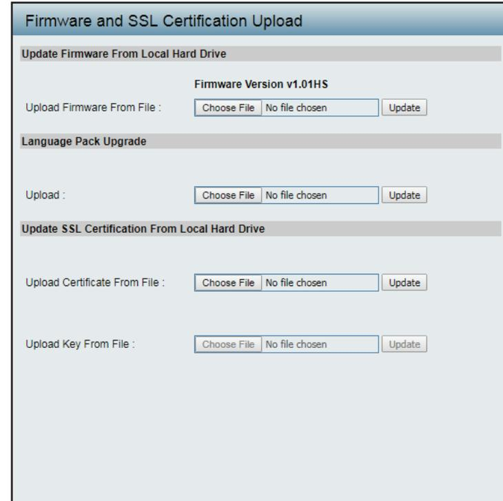
The screenshot displays a web interface titled "Firmware and SSL Certification Upload". It is divided into three main sections, each with a header bar:
