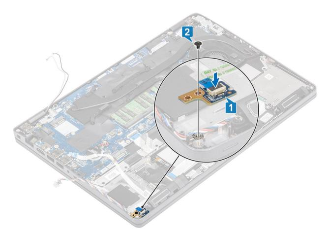
2 Connect the LED board cable to the system board and re-route it on the computer chassis [1,2]
