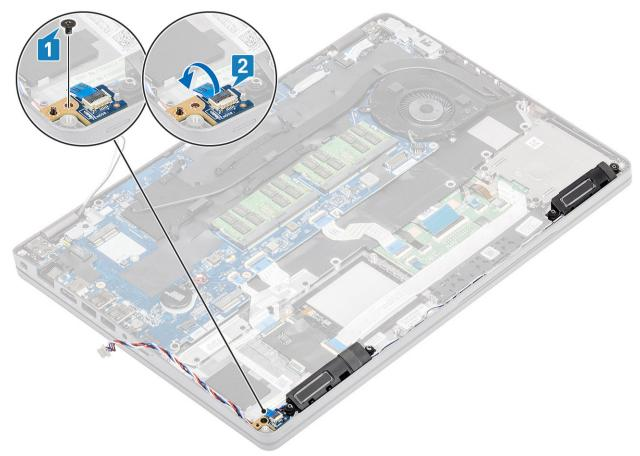
3 Un-route the speaker cables from the routing clips on the computer chassis.
