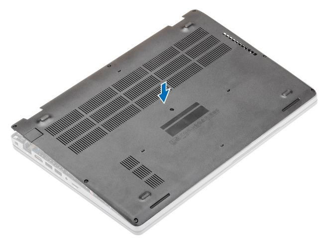
2 Press down on the edges pf the base cover till clicks in place.
