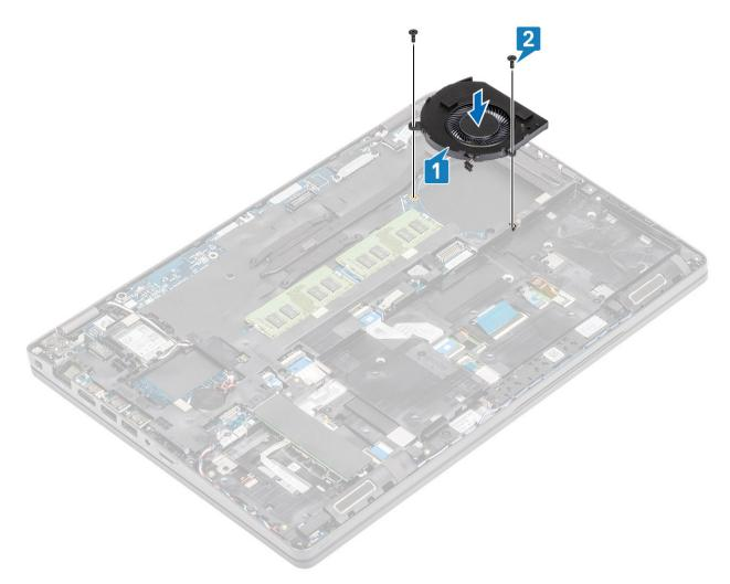
3 Connect the system fan cable to the connector on the system board.
