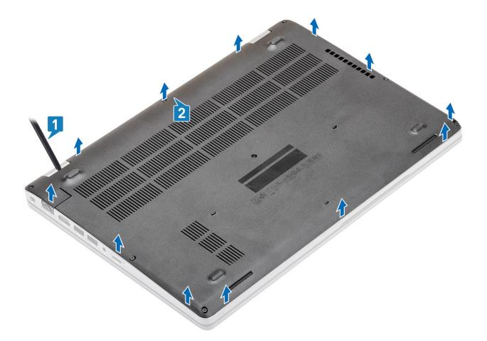
1 NOTE: While removing the base cover, on-site technicians must take care to remove the base cover carefully. There are prying recess points next to the left and right hinges which ease the disassembly procedure. With the help of a plastic scribe, pry open from the top left side of the base cover, continue working your way around the left and right side of the base cover, then remove the base cover from the system.
