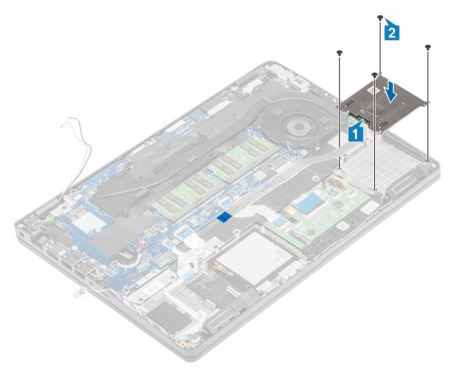
3 Re-connect the smart card reader cable to the system board and secure the cable to the computer [1,2].
