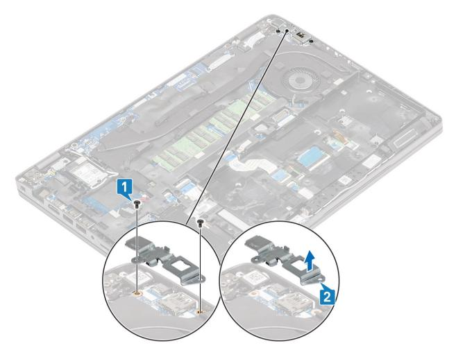
3 Disconnect the DC-in port cable from the connector on the system board and remove it from the computer [1,2].
