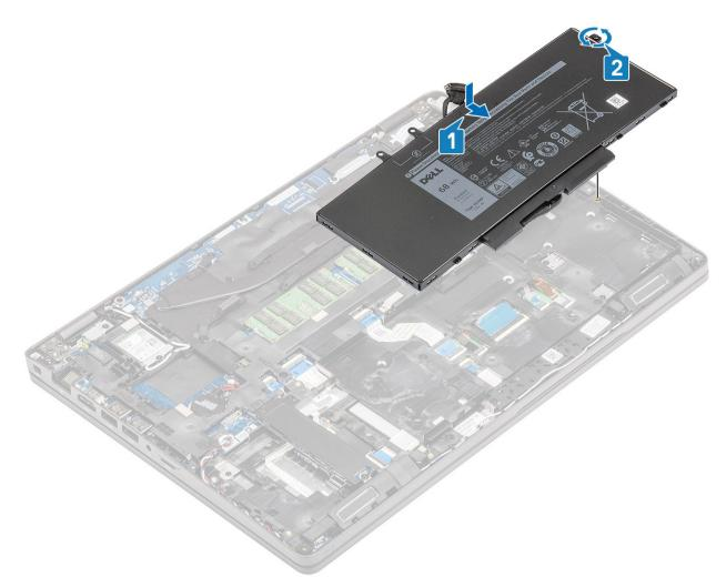
2 Reconnect the battery cable to the connector on the system board.
