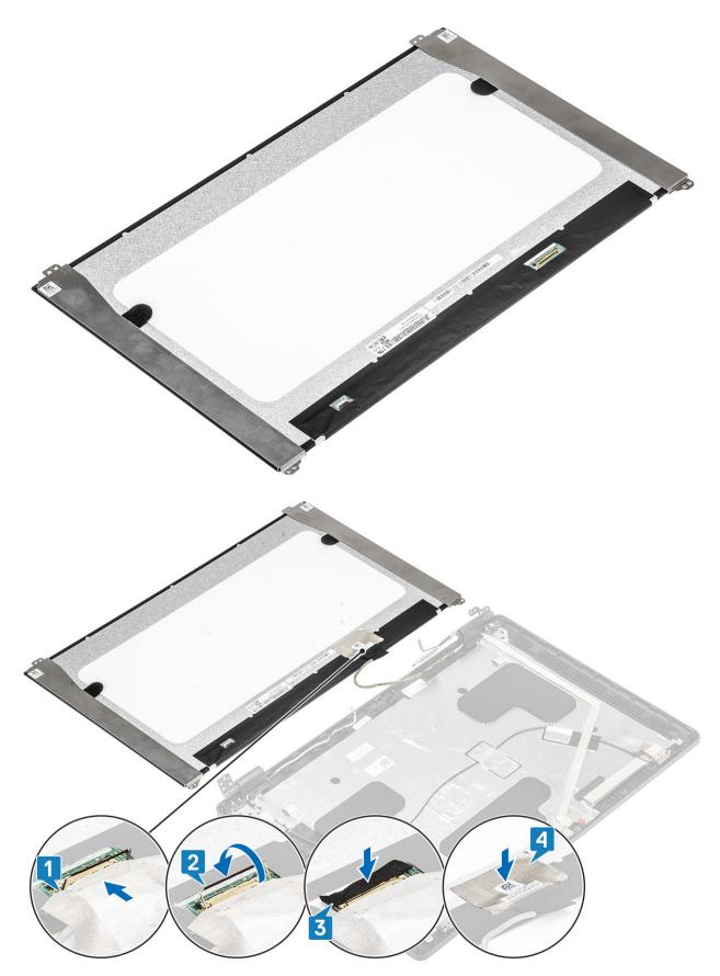
4 Replace the four (M2x2) screws that secure the display panel to the display assembly.
