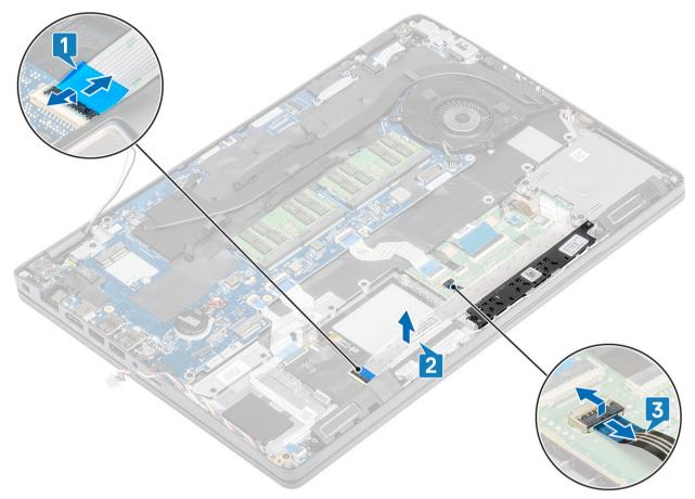
3 Remove the two (M2x3) screws and left the touchpad away from the computer [1,2].
