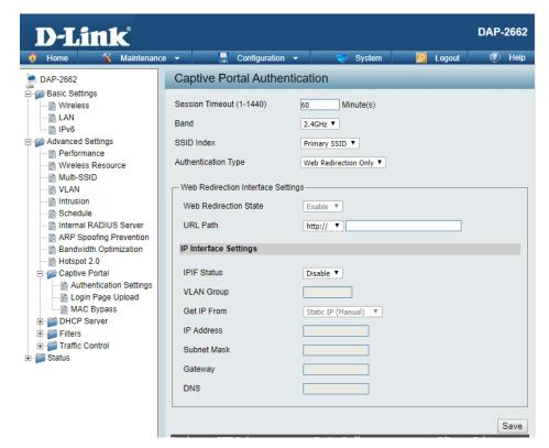
**IP Address:** Assign a static IP address that is within the IP address range of your network.
