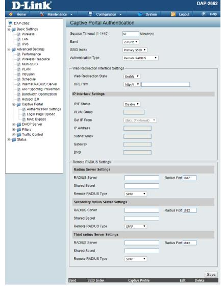
**IP Address:** Assign a static IP address that is within the IP address range of your network.
