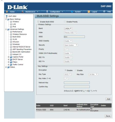
**Encryption:** When you select Open System, toggle between Enable and Disable. If Enable is selected, the Key Type, Key Size, Key Index
