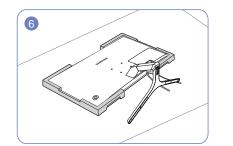
Install the COVER-REAR SUB after the power supply and the data cable are connected.
