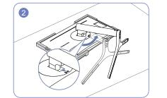
Push the key upward and hold. Turn the stand neck of the display counterclockwise for 10°.
