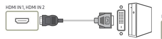
The audio function is not supported if the source device is connected using the HDMI-DVI cable.
