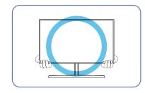
• Hold the lower corners or edges of the monitor when moving it.
