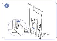
Open the COVER-STAND NECK LEFT, and rotate the open part at the bottom.
