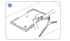
To disassemble the stand from the monitor, make sure to press the lower part of the monitor with one hand, and pull and sway sideways the stand with the other hand, as shown in the picture.
