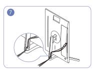
Place the corresponding cables into the stand-neck holder. Do not stretch the line. Three cables in one holder is recommended.
