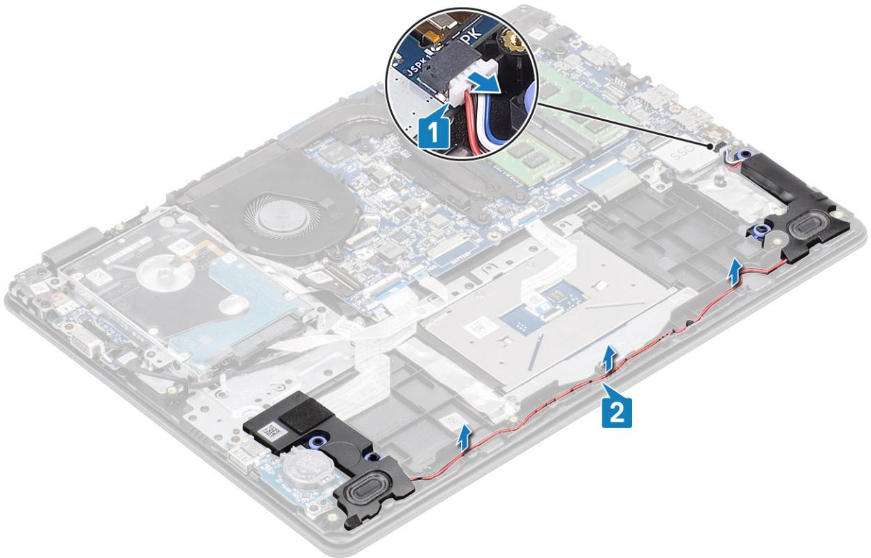
3 Lift the speakers, along with the cable, off the palm rest and keyboard assembly.
