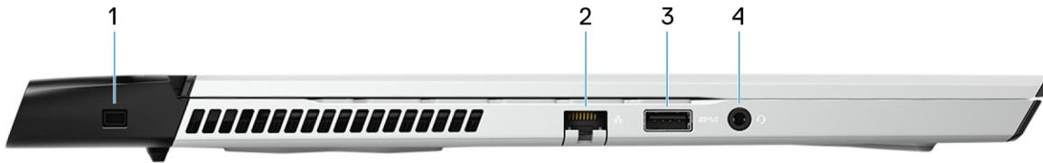
1 **Security-cable slot (wedge-shaped)**
