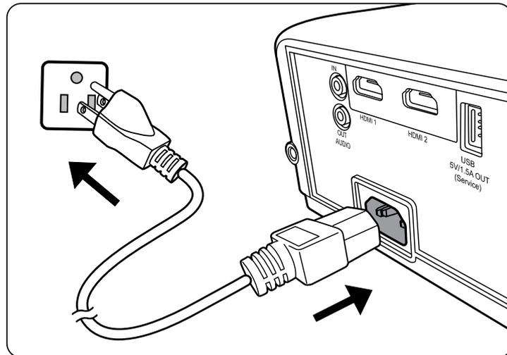
**NOTE:** When installing the projector, incorporate a readily accessible disconnect device in the fixed wiring, or connect the power plug to an easily accessible outlet near the unit. If a fault should occur during operation of the projector, use the disconnect device to switch off the power supply, or disconnect the power plug.
