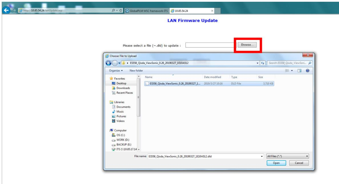
**iii.** After finishing the LAN Firmware update, please go to **Crestron e-Control®** page and click the “info” button to check the LAN Firmware version.
