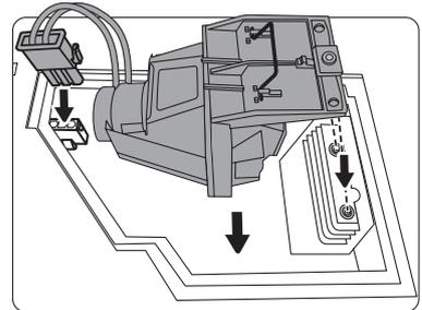
9. Insert the lamp connector and tighten the screw that secures the lamp.
