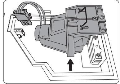
8. As show in the figure, insert the new lamp. Align the lamp using the alignment holes and gently push the lamp into the locked position
