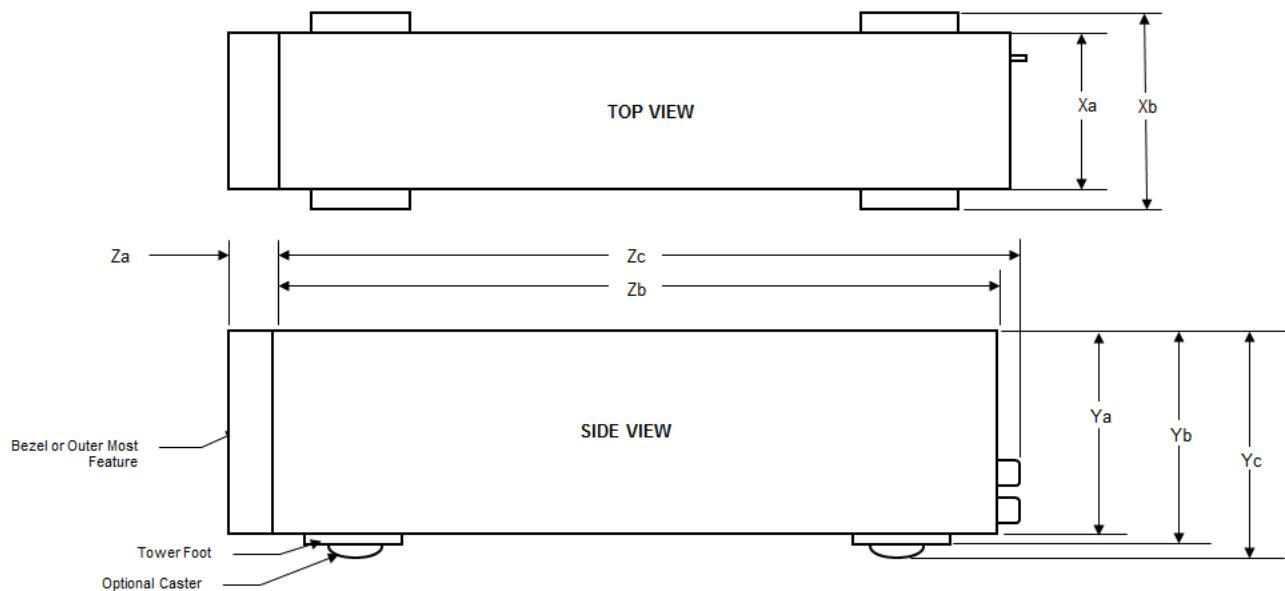
Figure 1. Dell EMC PowerEdge T440 system dimensions
