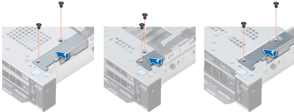
Figure 117. Installing the cable cover
