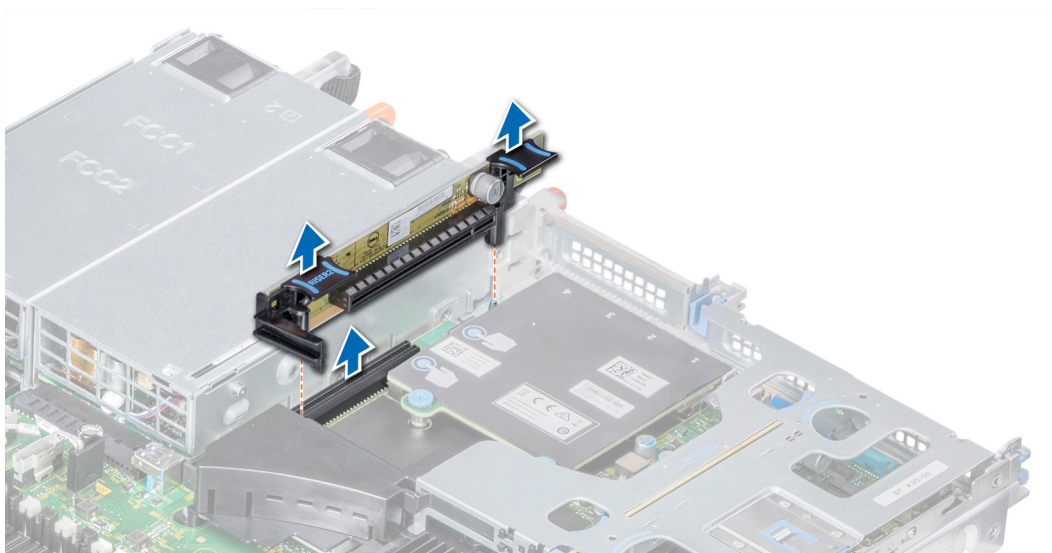
Figure 48. Removing the expansion riser 2A
