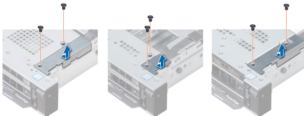
Figure 114. Removing the cable cover
