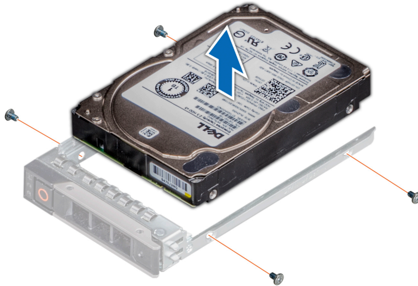
Figure 79. Removing the drive from the drive carrier
