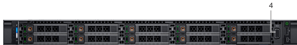
Figure 4. Front view of 10 x 2.5 inch drive system
