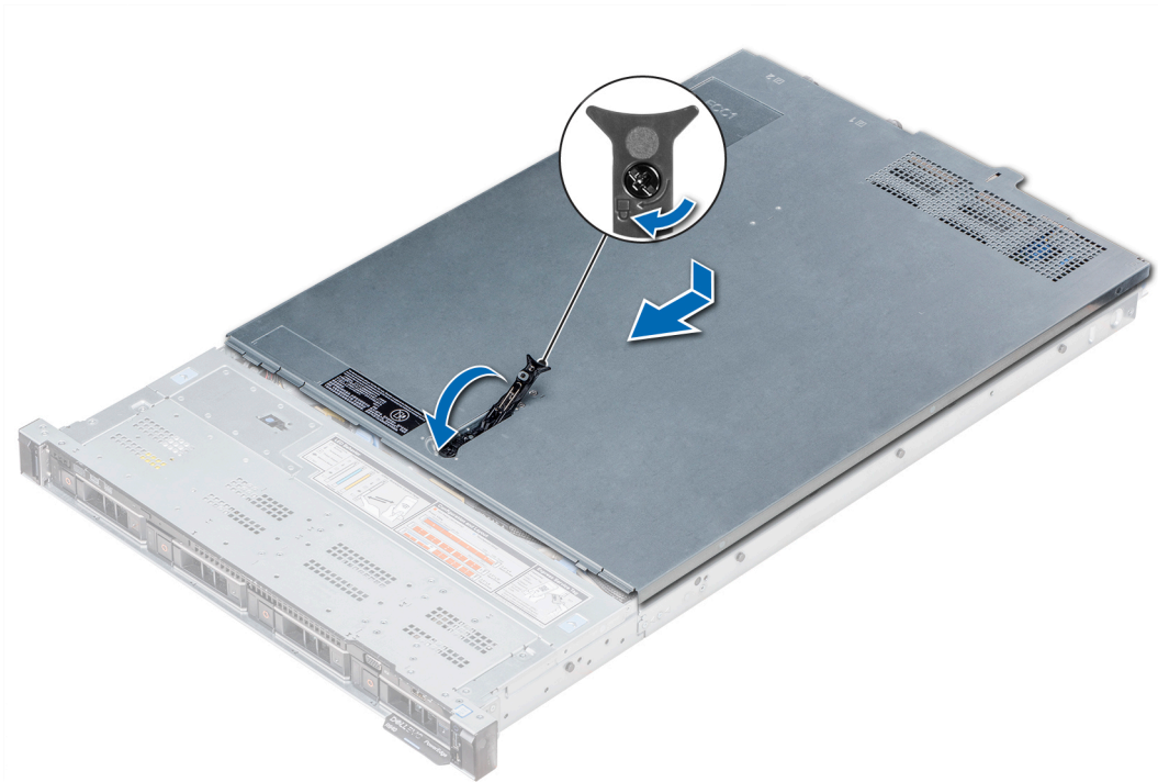
Figure 24. Installing the system cover
