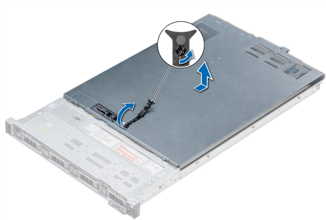
Figure 23. Removing the system cover
