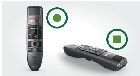
Being on the cutting edge of technology, the SpeechMike Premium Air comes with an integrated motion sensor, meaning it can be controlled by the movement of your hand. It detects when it's put on the table, mutes the microphone, and once it is being picked up again it unmutes the microphone. In addition to that, custom events can be programmed, e.g., to pause and to continue the recording.
