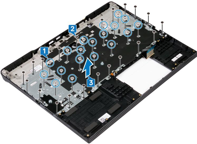
4 Lift the keyboard, along with its cable, off the palm-rest assembly.
