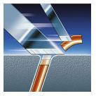
The dual blade system of this electric shaver lifts hairs to cut comfortably below skin level.
