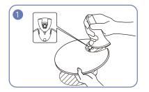
Insert the stand neck into the stand base in the direction shown in the figure. Check that the stand neck is firmly connected.
