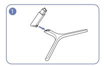
Insert the stand neck into the stand base in the direction shown in the figure. Check that the stand neck is firmly connected.
