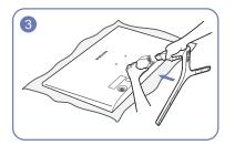
Place a soft cloth over the table to protect the product and place the product onto the cloth so that the front of the product is facing downwards. Hold the back of the monitor as shown in the figure. Push the assembled stand into the main body in the direction of the arrow as shown in the figure.
