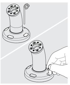
Fixing From Above: Lift & hold the rubber screw covers. Use caution to not scratch the parts.
