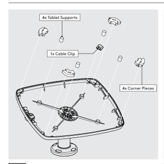
Install the Tablet Setup Kit. Each kit is specific per tablet device and Bouncepad Case.
