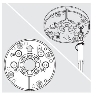
Configure the angle of rotation - ensuring both arrows are pointing in the same direction before starting. Default angle configuration is 270°. Insert the limit screws for 90° or 180° rotation.
