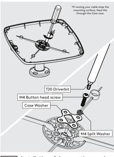
Installation of the mounting arm is complete. Now install your Case as shown above.
