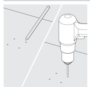
Using the template (see A4) mark and drill the mounting holes appropriate to your mounting surface and cable routing configuration.
