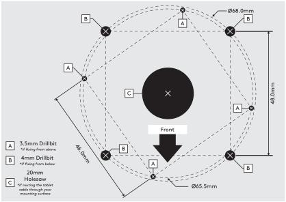
Use the above template to mark the drill holes - appropriate to your chosen fixing method. 'A' if fixing from above. 'B' if fixing from below. Follow the corresponding steps (PTO) specific to each fixing method.
