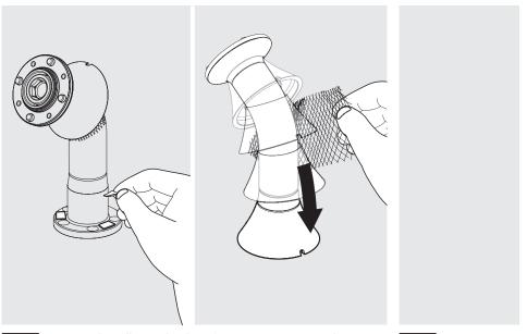
Remove the adhesive backing & protective netting, then locate the Stalk Cover to the mount surface. Installation is complete.
