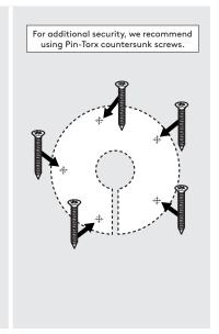
Remove the adhesive backing & protective netting, then locate the Stalk Cover to the mount surface.
