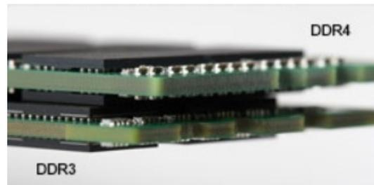
**Figure 2. Thickness difference**
