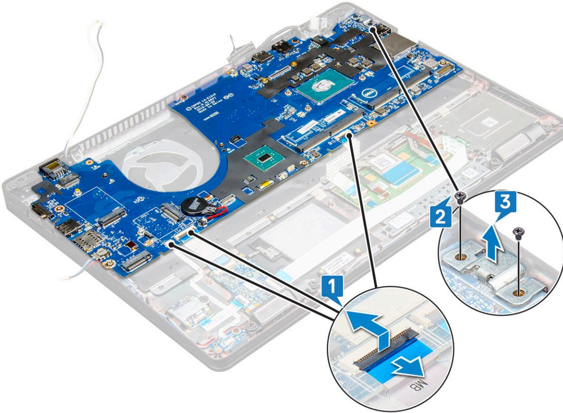
5 Remove the M2.0x3.0 screws (3) and lift the system board away from the computer [1, 2].
