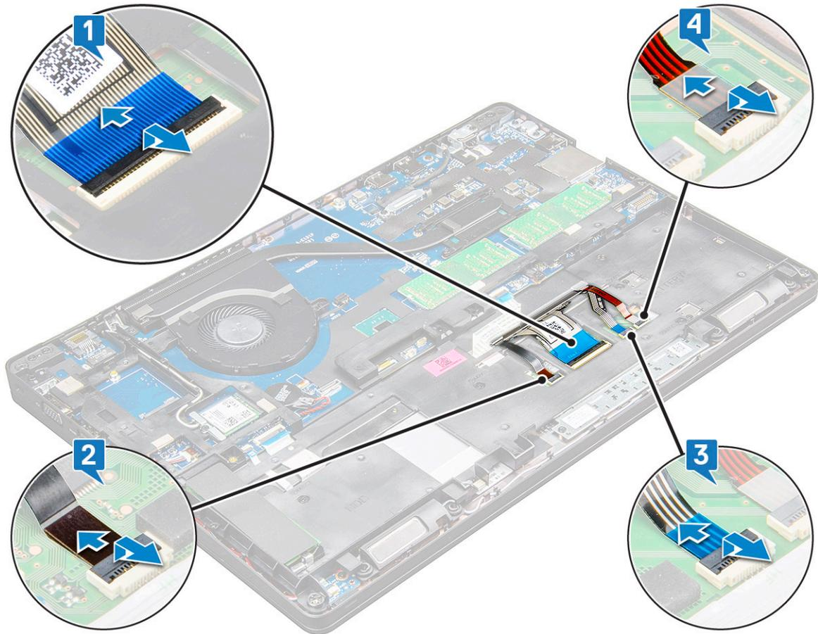
c Lift the latch and disconnect the cable from the connector on the system board [3].
