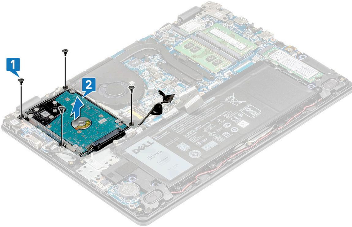
4 Disconnect the HDD cable interposer.
