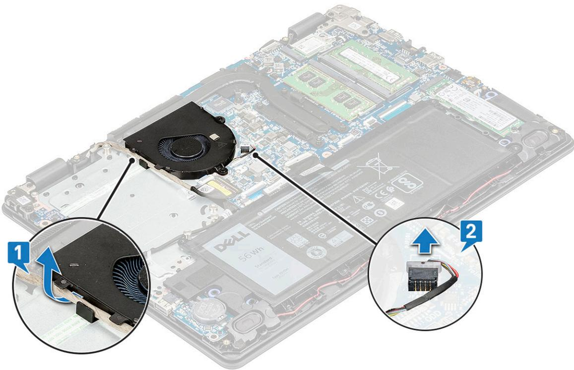
b Remove the 2 M2.5x5 screws that secure the fan to the computer [1] and lift the fan off the computer [2].
