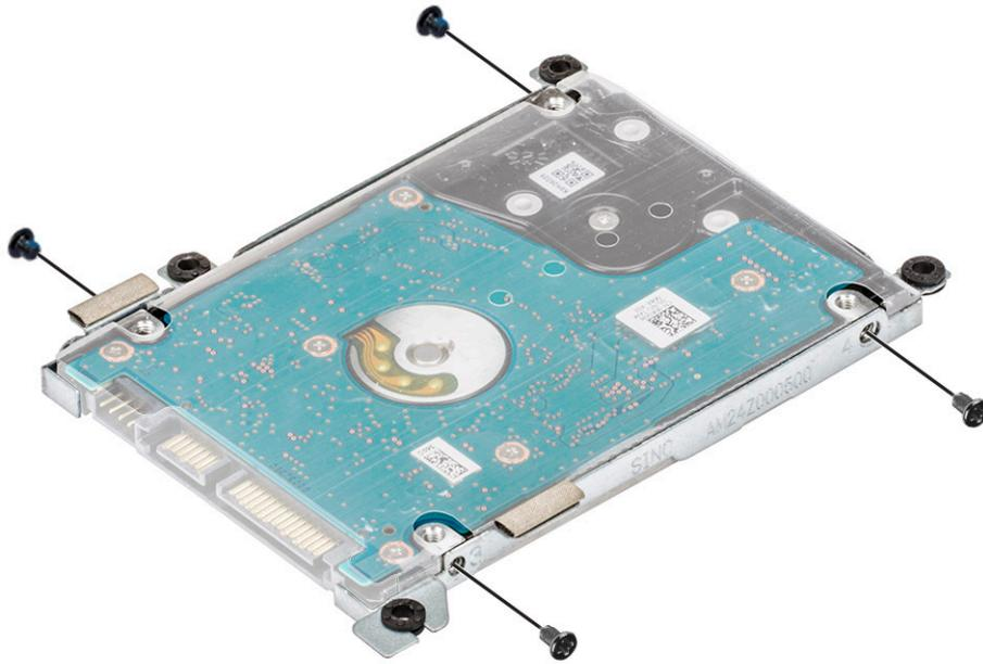
6 Lift the HDD bracket to remove it from the HDD.
