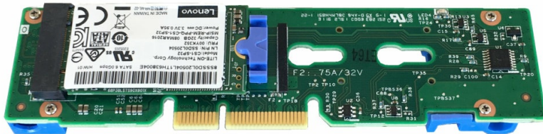
Figure 12. ThinkSystem M.2 Enablement Kit (shown with an 32 GB M.2 drive, not supported in the SE350)
