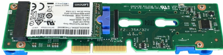
Figure 12. ThinkSystem M.2 Enablement Kit (shown with a 32 GB M.2 drive, not supported in the SE350)
