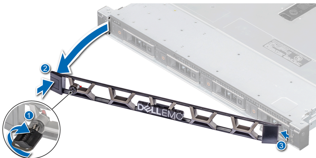
Figure 9. Removing the front bezel
