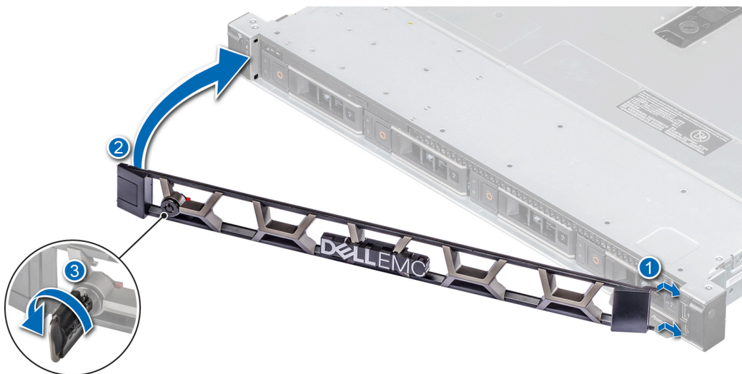
Figure 10. Installing the front bezel
