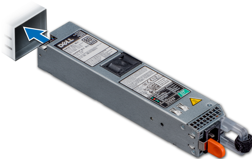
Figure 71. Installing a power supply unit
