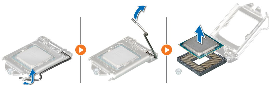
Figure 52. Removing the processor
