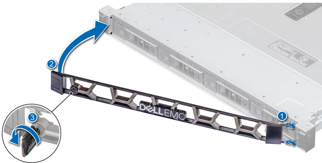
Figure 14. Installing the optional front bezel
