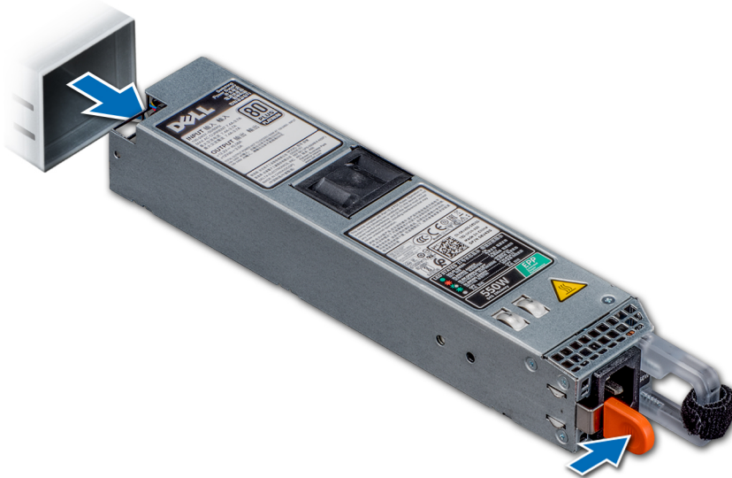
Figure 70. Removing a power supply unit
