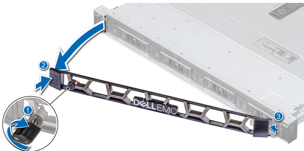
Figure 13. Removing the optional front bezel
