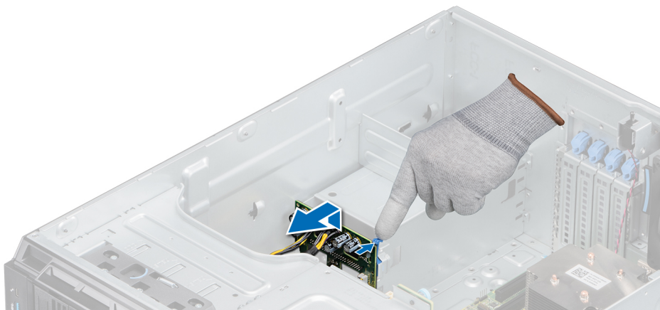
Figure 76. Removing the power interposer board
