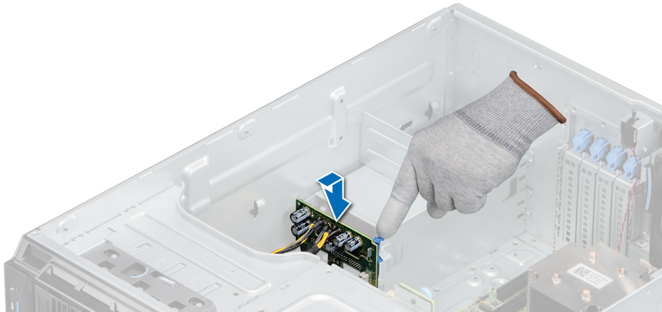
Figure 77. Installing the power interposer board
