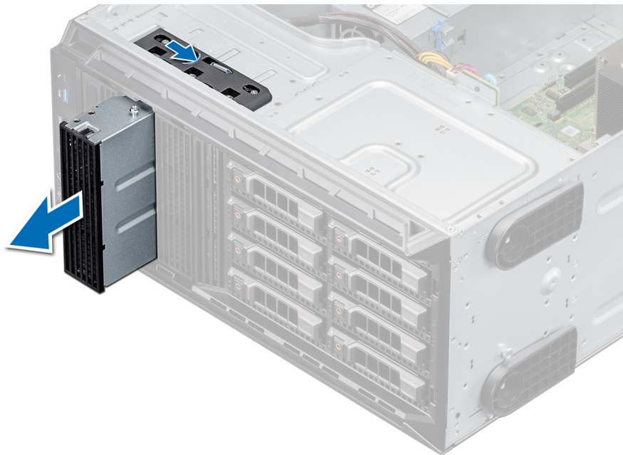
Figure 38. Removing the optical drive or tape drive blank
