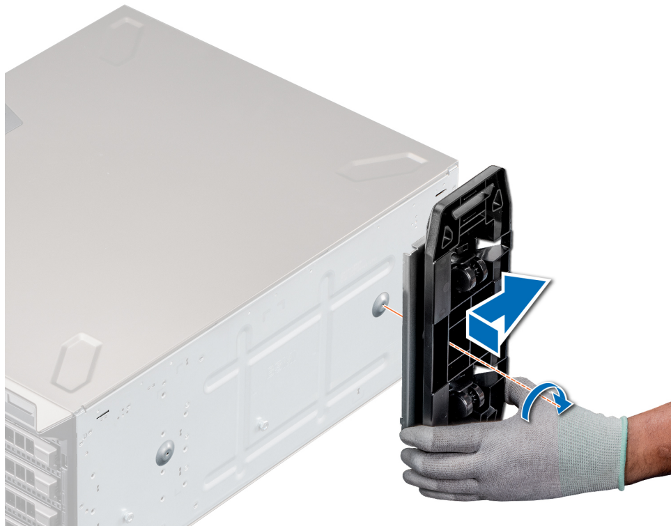
Figure 21. Installing caster wheels
