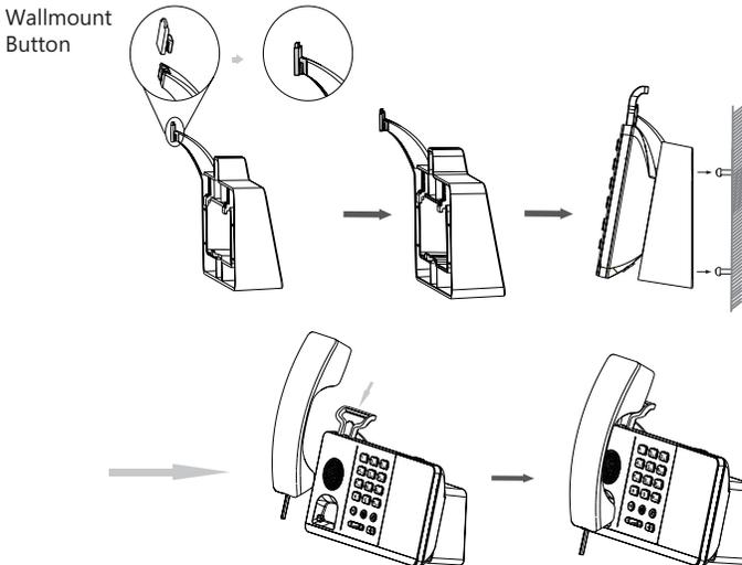
**Note:** You need to attach the wallmount button to the wallmount bracket first to hook the handset and prevent it from slipping.
