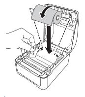
For fanfold paper Insert the fanfold paper as shown in the illustration.
