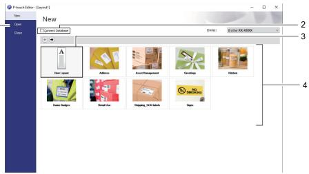
To change how P-touch Editor starts, click **Tools** > **Options** in the P-touch Editor menu bar to display the **Options** dialog box. On the left side, select the **General** heading, and then the setting you want in the **Operations** list box under **Startup Settings**.
