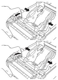
5. Insert the roll so that the label print side is facing up, as shown in the illustration.
