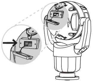
5. Push and hold the reset button for more than 8 seconds. The red LED indicator on the PCBA board will come on to show that the hardware reset started.
