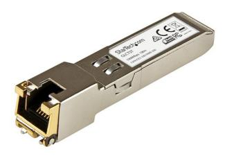
The 10050-ST is an Extreme Networks 10050 compatible copper transceiver module that has been designed, programmed and tested to work with Extreme Networks brand switches and routers. It delivers dependable 1 GbE connectivity over copper cable, for 1000BASE-T compliant networks, with a maximum distance of up to 100 m (328 ft).
