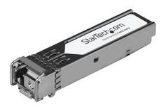
The 10057-ST is an Extreme Networks 10057 compatible upstream fiber SFP transceiver which pairs with StarTech.com's 10056-ST. They are designed, programmed and tested to work with 1000BASE-BX-U compatible Extreme Networks switches and routers. The SFP transceiver module supports a maximum distance of up to 10 km (6.2 mi) and delivers dependable 1 GbE connectivity over fiber cabling.
