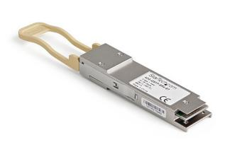
The 40G-QSFP-SR4-ST is a Brocade 40G-QSFP-SR4compatible fiber transceiver module that has been designed, programmed and tested to work with Brocade brand switches and routers. It delivers dependable 40 GbE connectivity over fiber cable, for 40GBASE-SR4 compliant networks, with a maximum distance of up to 150 m (492 ft.).
