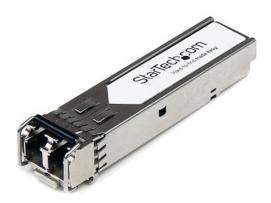
The 455886-B21-ST is a HPE 455886-B21 compatible fiber transceiver module that has been designed, programmed and tested to work with HPE brand switches and routers. It delivers dependable 10 GbE connectivity over fiber cable, for 10GBASE-LR compliant networks, with a maximum distance of up to 10 km (6.2 mi).
