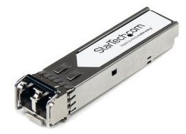
The EW3B0000710-ST is a Citrix EW3B0000710 compatible fiber transceiver module that has been designed, programmed and tested to work with Citrix brand switches and routers. It delivers dependable 10 GbE connectivity over fiber cable, for 10GBASE-SR compliant networks, with a maximum distance of up to 300 m (984 ft).
